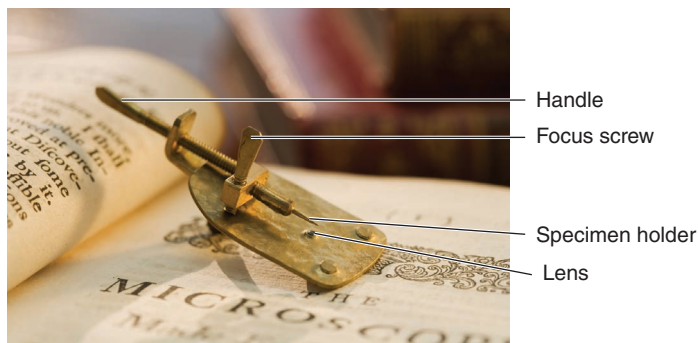
FIGURE 1.1 Model of van Leeuwenhoek's Microscope The original made in 1673 could magnify the object being viewed almost 300 times. The object being viewed is brought into focus with the adjusting screws. Note the small size.
